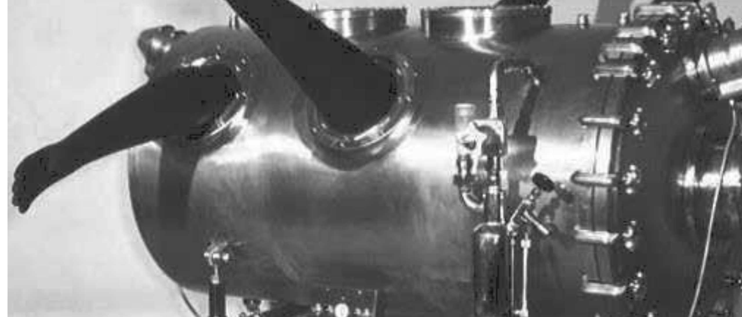
Steam sterilizable metal isolator (Notre Dame University, 1928)
